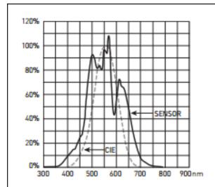
Characteristic curve showing the sensor's sensitivity in respect of the wavelength of light. The broken line represents the light perception of the human eye
