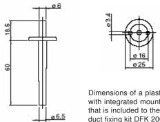
Dimensions of a plastic tube with integrated mounting plate, duct fixing kit DFK 200
